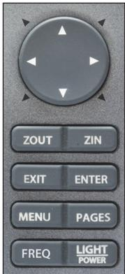
**Arrow Keypad** Activates cursor on Sonar page. Press up, down, left or right to move the cursor.
